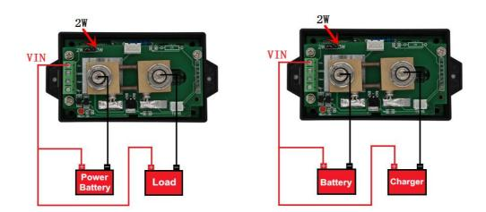
The above figure applies to VAT1050, VAT1100, VAT1200, VAT1300 measurement circuit voltage of 10-100V; attention at this time attention to the jumper cap to receive 2W, the left wiring method is suitable for battery discharge measurement and DC circuit measurement; The wiring method on the right is only suitable for charging the battery.
