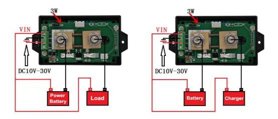
The figure above applies to batteries or circuits where the VAT4300 measures 0-400V and VAT1050, VAT1100, VAT1200, and VAT1300 to 0-100V; at this time, note that the jumper cap must be connected to 3W and need to use a 10-30V. The DC voltage supplies power to the measurement module; the wiring method on the left is suitable for the discharge measurement of the battery and the measurement of the DC circuit; the wiring method on the right is only suitable for the charge measurement of the battery.
